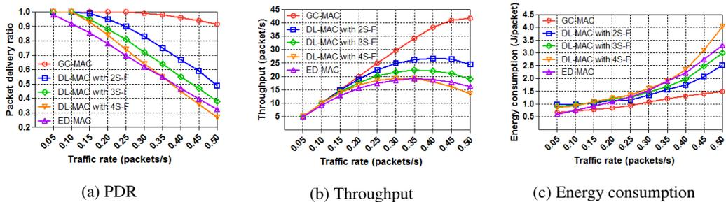
Figure 1: Shallow region scenario: PDR, Throughput, and Energy consumption vs. Traffic rate.
